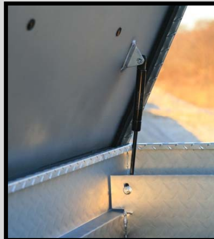
Reinforced Foam Filled Lid with Heavy Duty Gas Shocks
