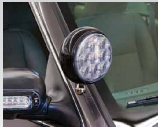
P46SLC shown mounted in Unity spotlight assembly.
