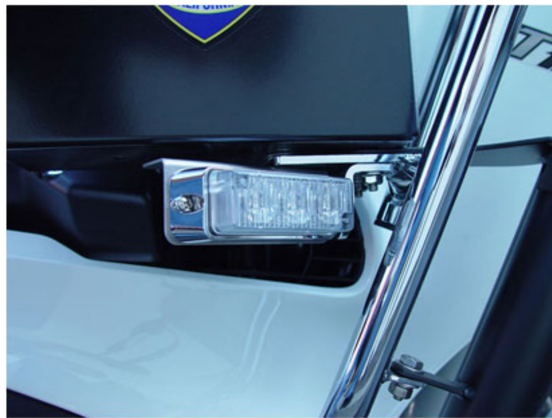
TIR3 - Passenger side Front warning All LED's are High Intensity Super LED
