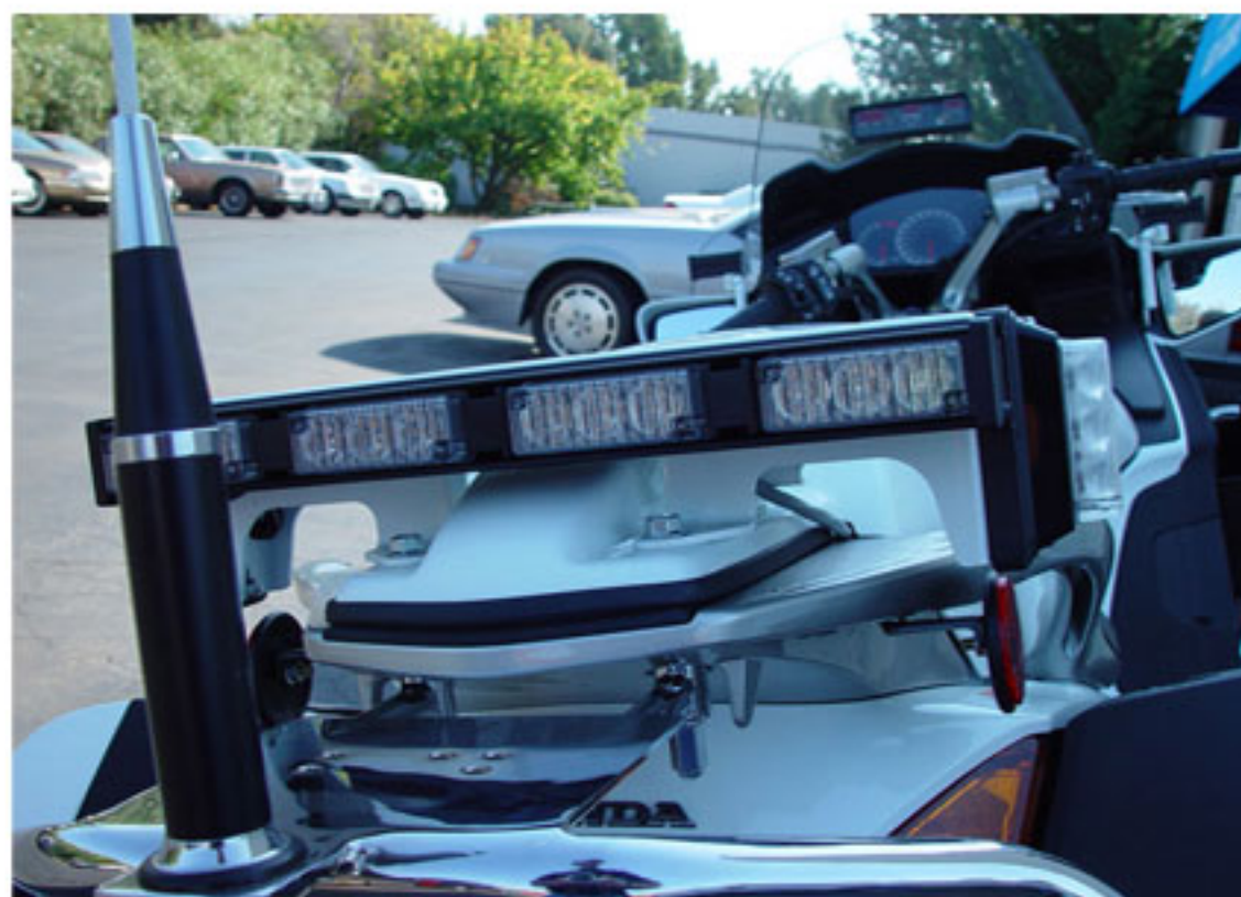
Verticle Mount TIR3 for Side Protection w/ Optional Dominator 4
