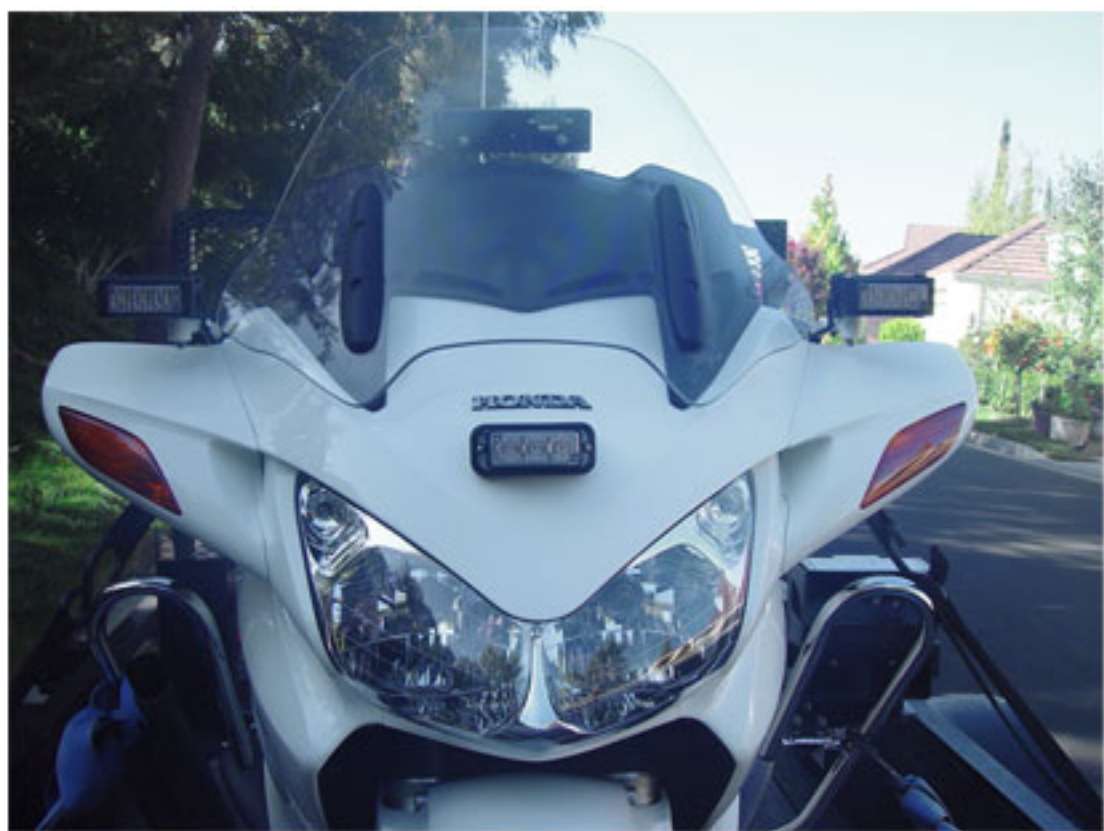
Dominator 1 LED post mounts w/ center CA Steady Red
