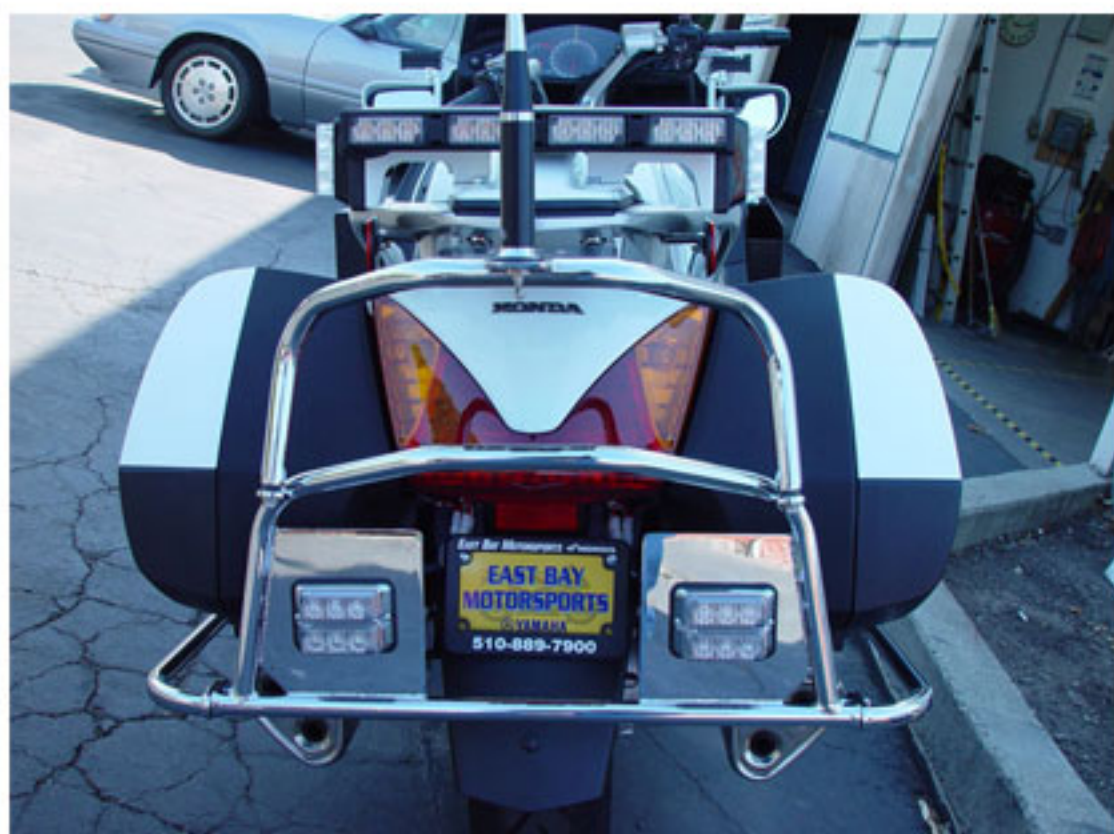
Upper Rack Dual TIR3 Mounted to Crash Bar w/ Optional Dominator 4
