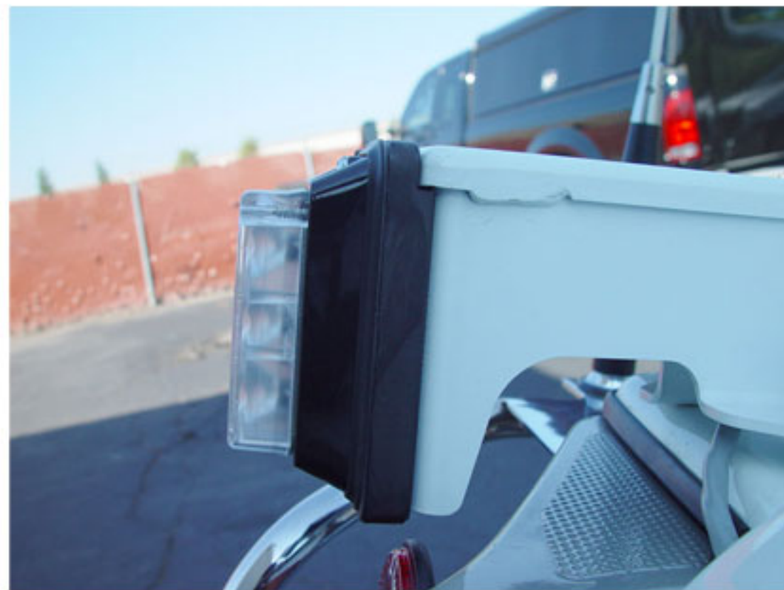
Custom Verticle Mount TIR3 to attach to Honda Rear Bracket
