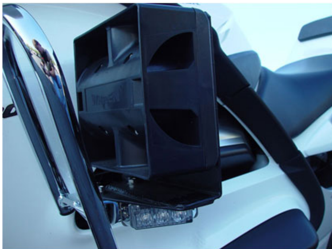
SA314P Siren Speaker with TIR3 LED for front driver's side warning
